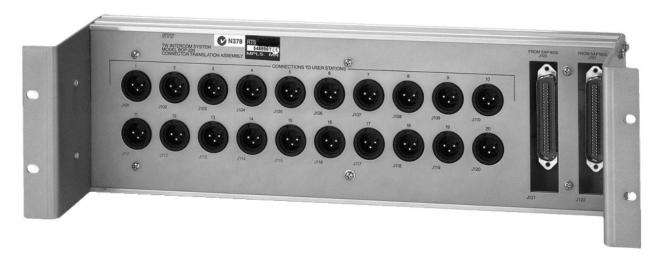
19", 3 **RU** (Rack Unit) breakout panel, I/O connector transition assembly. Provides a convenient interface between a SAP-1626 (25-pair 50-pin) and up to 20 user stations or strings of stations (3-pin XLR male).
