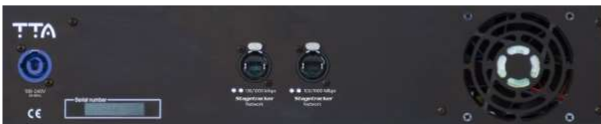
Figure 4 Stagetracker II™ Net unit, rear panel
