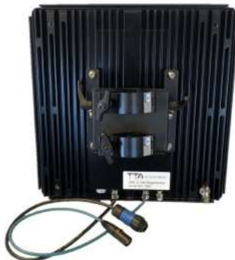
Figure 6 RadioEye mounting bracket and cable connections.
