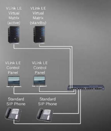
The **VLink LE Virtual Matrix**, the central brain of the system, is a server-software based equivalent of an RTS hardware matrix. In the same way most hardware systems support redundant master controllers, the VLink LE system supports a duplicate stand-by server that takes over if the active server fails.
